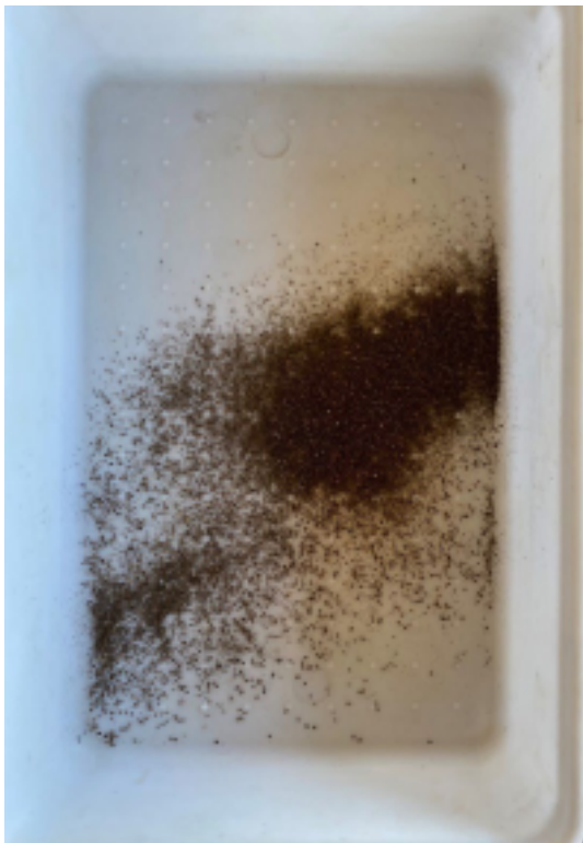
Figure 8. Soil passed through 2mm screen
