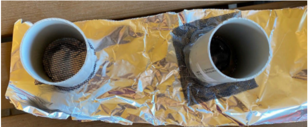
Figure 3. Gluing Mesh to PVC Pipe on Foil
