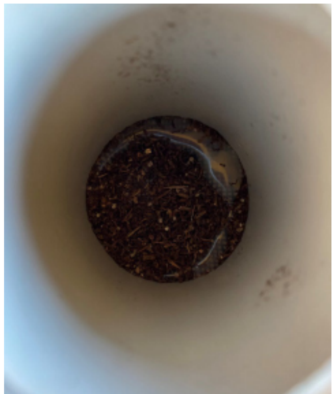
Figure 9. Soil passed through 2mm screen was placed on 1mm screen
