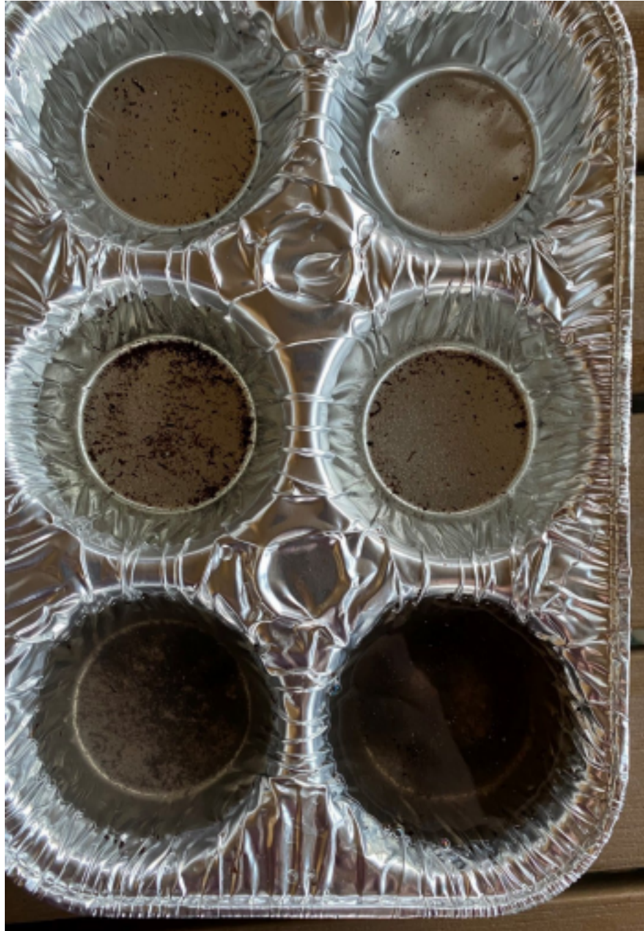
Figure 14. The soil particles in the top muffin cups are particles that passed through the screen during the capillary rewetting process. In the middle cups, the unstable aggregates that passed through the screen during wet sieving. The bottom cups contain stable aggregates that were collected after treating the aggregates with dish soap and breaking up the stable aggregates.
