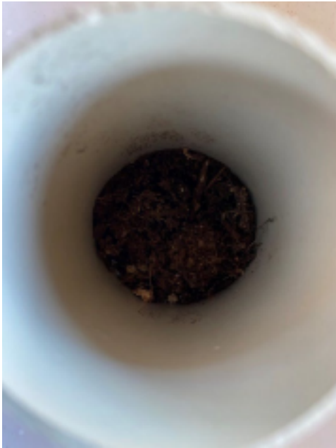
Figure 6. Soil placed on 2mm sieve
